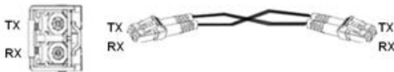
Figure 10 Cable Connection of Gigabit SFP Optical Module
