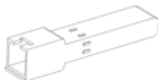
Figure 12 Gigabit SFP Electrical Module
