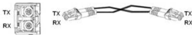
Figure 18 Fiber Connection of an SFP Optical Module
