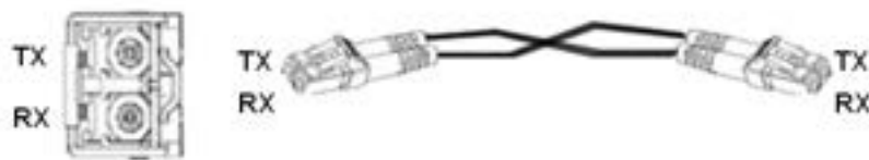
Figure 8 Fiber Connection of an SFP Optical Module
