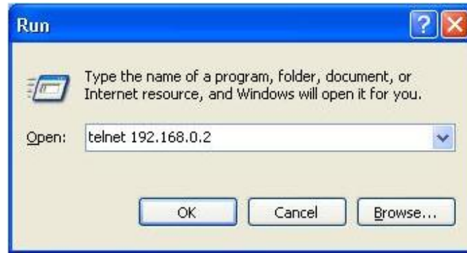
Figure 19 Access through Telnet
