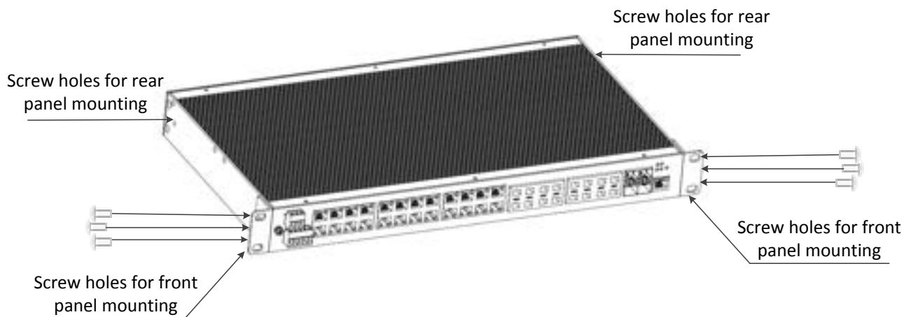
Figure 4 Installing Mounting Brackets
