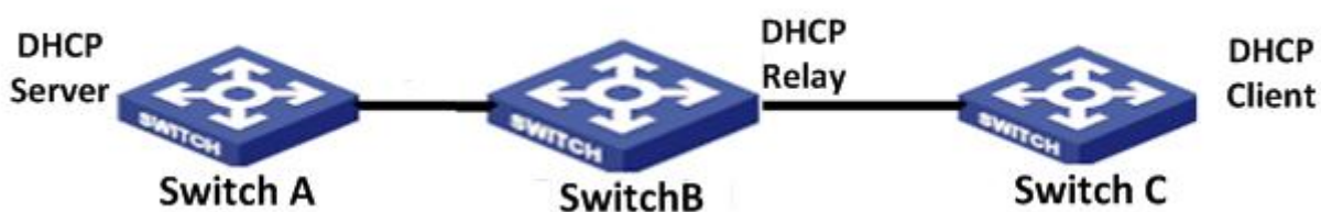
Figure 196 DHCP Typical Configuration Example
