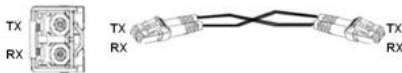
Figure 7 Fiber Connection of an SFP Optical Module
