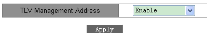
Figure 327 Enabling TLV Management Address
