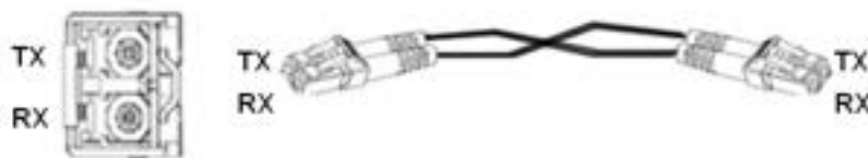
Figure 9 Fiber Connection of an SFP Optical Module
