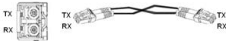
Figure 10 Fiber Connection of an SFP Optical Module
