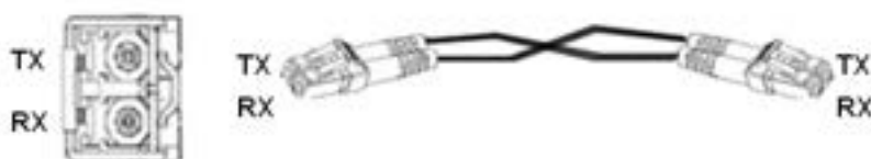
Figure 16 Cable Connection of 100M SFP Optical Module
