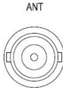
Figure 12 SAT Antenna Interface
