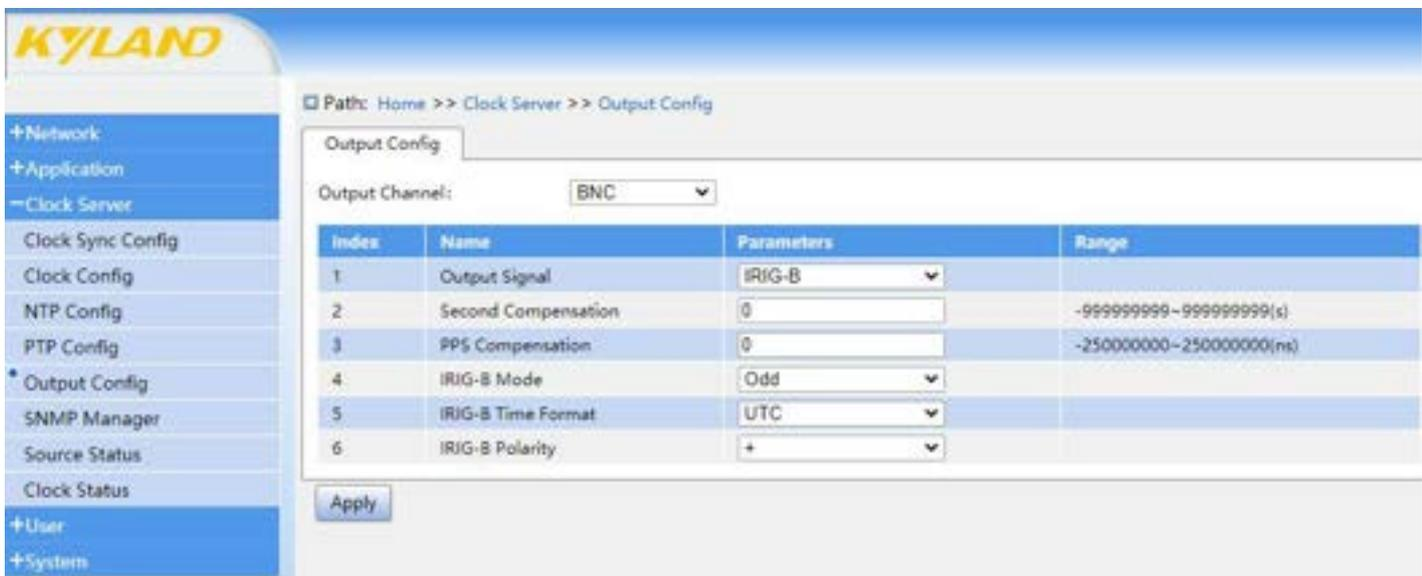
Figure 41 BNC Channel Output Parameters
