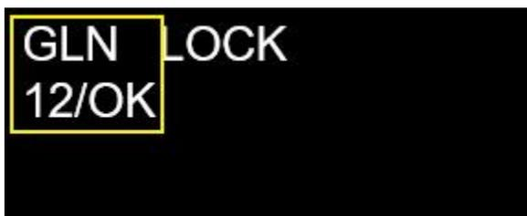
Figure 76 Synchronization source status: GLONASS
