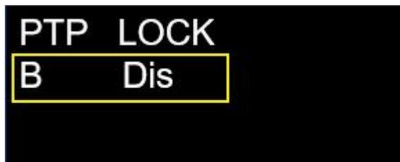
Figure 79 Synchronization source status: PTP Boundary clock, Dis
