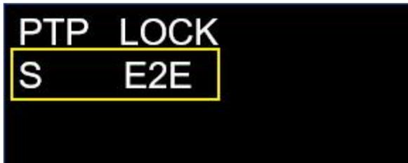
Figure 78 Synchronization source status: PTP Slave clock, E2E
