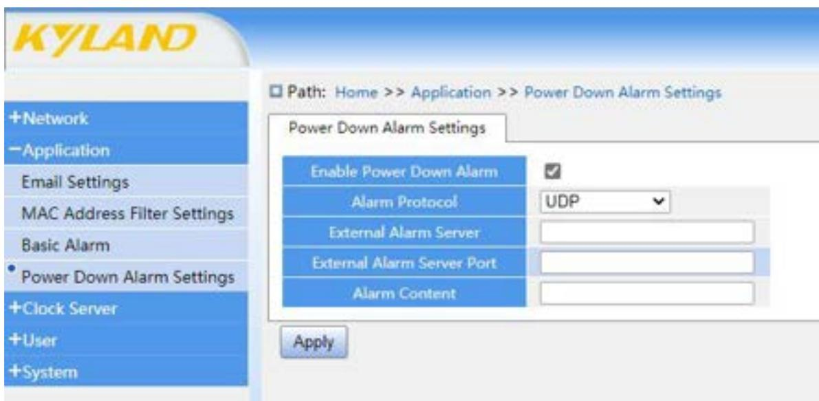
Figure 13 Power-down Alarm
