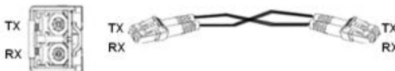
Figure 5 Fiber Connection of an SFP Optical Module
