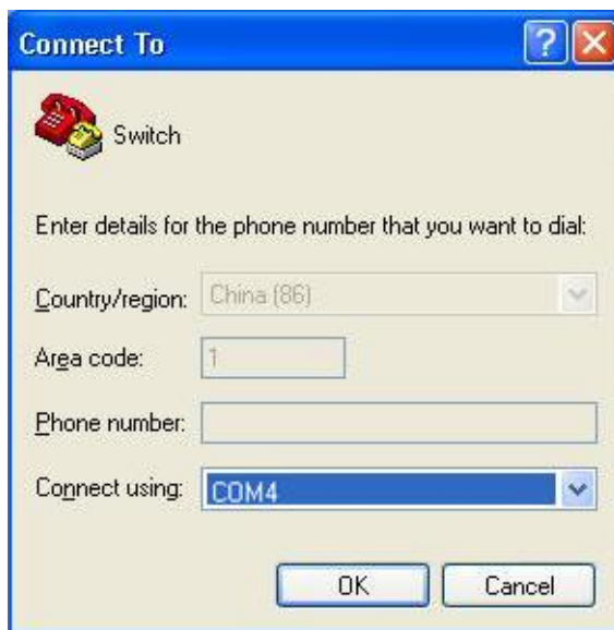
Figure 14 Selecting the Communication Port in Use
