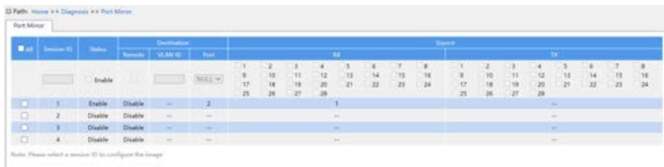
Figure 235 Configure Port Mirror Function
