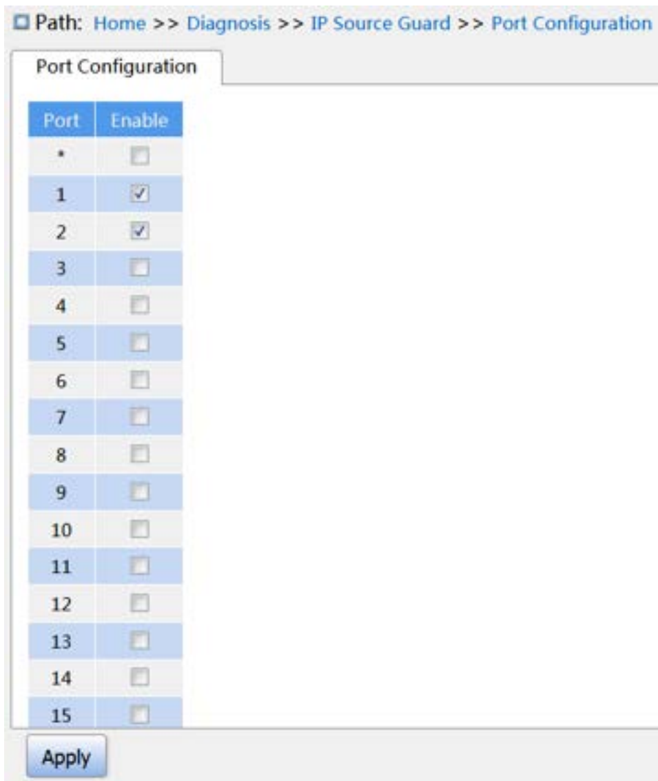
Figure 246 Configure Port IP Source Guard
