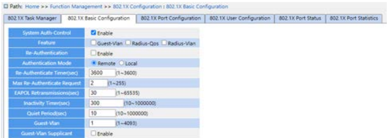
Figure 199 IEEE802.1X Basic Configuration
