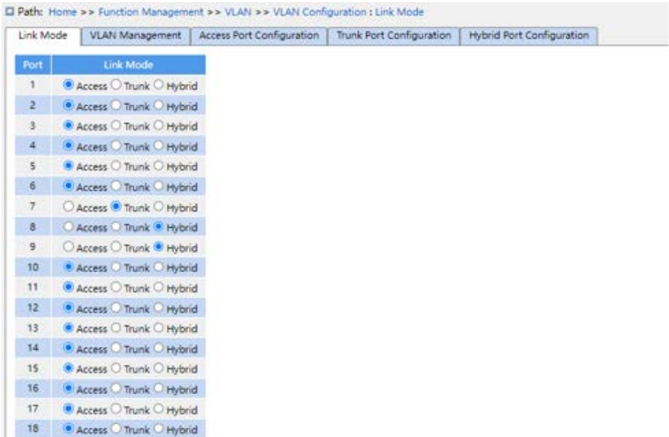
Figure 97 configurate port link mode
