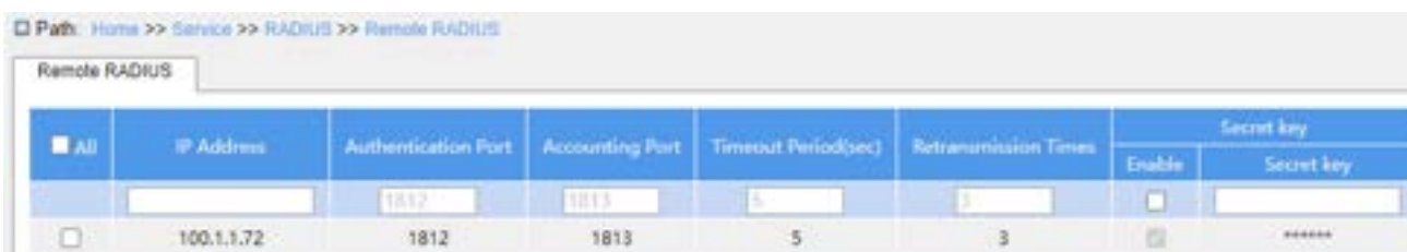
Figure 69 Configure the RADIUS Server
