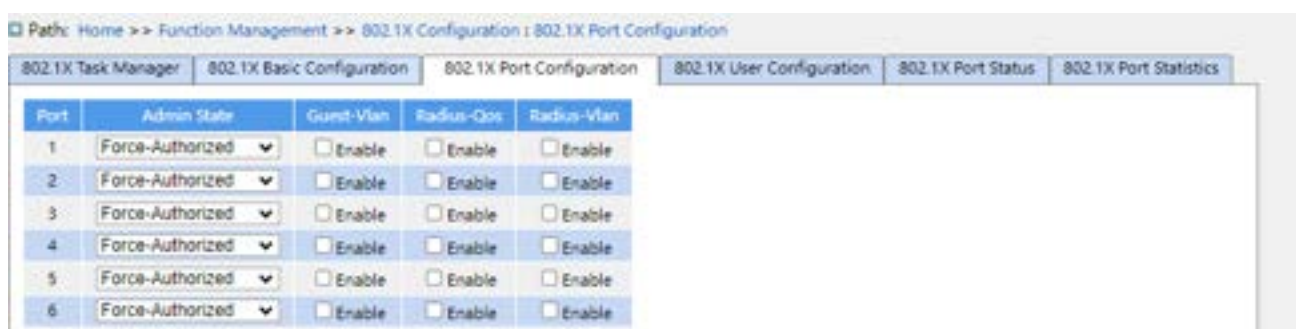
Figure 200 Configure IEEE802.1X port
