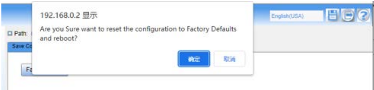
Figure 16 Restore the factory configuration
