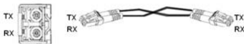
Figure 13 Fiber Connection of an SFP Optical Module
