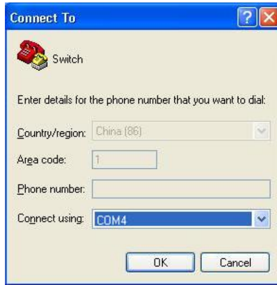
Figure 20 Selecting the Communication Port in Use
