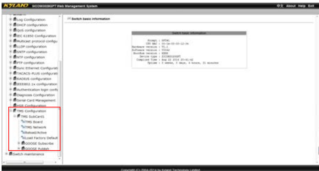
Figure 3 The Navigation Tree of TMS Configuration
